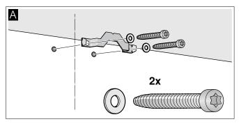
2 Screw on brackets for the extractor hood handtight. Do not fully tighten screws!
