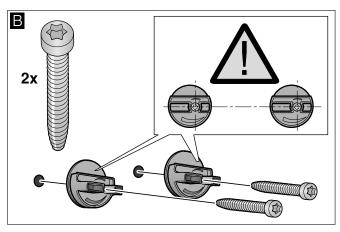
3 Screw in threaded bolt, leaving it protruding out of the wall by <sup>3</sup>/<sub>16</sub>" - <sup>11</sup>/<sub>32</sub>" (5−9 mm).
