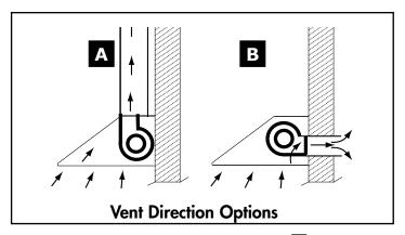
The factory default direction is through the **top** A of the hood. However, the blower can be rotated to vent through the rear B of the hood.
