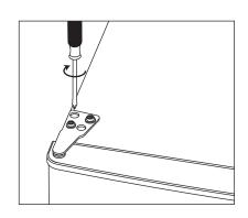
12 Re-attach the hinge cover and the screw cover.
