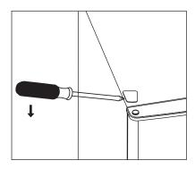
Move the hinge hole cover from the left side to the right side. Then lift the door and place it on a padded surface to prevent it from scratching.
