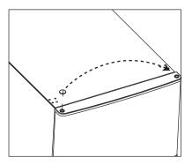
6 Remove the adjustable feet from both sides. Remove the screws and the bottom hinge.
