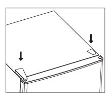
13 With the door closed, check that the door is aligned horizontally and vertically, and that the seals are closed on all sides before finally tightening the bottom hinge. Re-adjust the leveling feet as needed.
