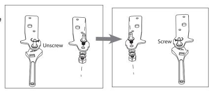
8 Re-attach the bottom hinge bracket on the left side. Re-attach both adjustable feet. Re-attach the lower door in the proper position, by fitting it on the hinge.
