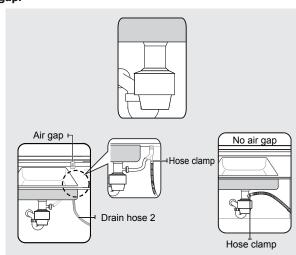
3. The drain hose molded end will fit 5/8", 3/4", or 1" diameter connections on the air gap, waster tee, or disposer. Cut on the marked line as required for your installation.
