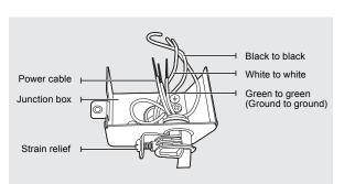
4. Connect the BLACK wire of the dishwasher to the BLACK wire of the power cable by inserting both into a wire nut and then rotating the wire
