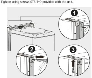
Secure dishwasher to the cabinet side wall if the countertop can be damaged by top mounting the unit. To attach the two installation brackets to the side of the dishwasher, remove the adjustment caps from the sides of the unit. Use pliers to snap off the end of the long leg of the bracket. Insert each bracket tab into the corresponding slot on the side of the dishwasher and tighten using screws ST3.5\*9 provided with the unit.
