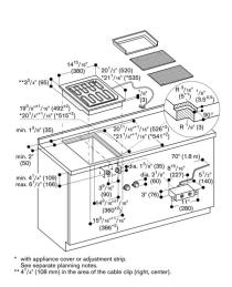
Installation with appliance cover/adjustment strip; surface installation
