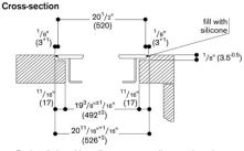
For installation with appliance cover or adjustment bar, observe the deeper notch and the slot width front and back.
