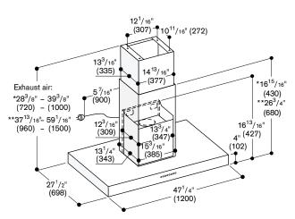
With the exhaust air duct cover AD 442 016 suitable for ceiling heights of 7.9 ft (2.35 m) to 8.6 ft (2.60 m).
