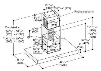
\* With the air recirculation duct cover AD 442 116 suitable for ceiling heights of 7.9 ft (2.35 m) to 8.6 ft (2.60 m).
