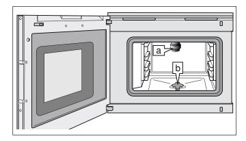
The cleaning program removes stubborn dirt. A cleaning cartridge (a) is screwed into the top of the cooking compartment. The cooking compartment is cleaned, rinsed, and dried completely automatically. The drain filter (b) must remain inserted in the cooking compartment floor while the cleaning program is in progress.
