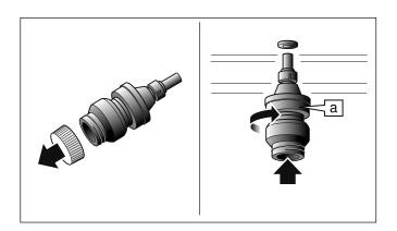
6 Screw the descaling cartridge (a) into the socket in the top of the cooking compartment up to the stop. Close the appliance door. Press ✓ to confirm. A descaling time of 2 hours 15 minutes is displayed.
