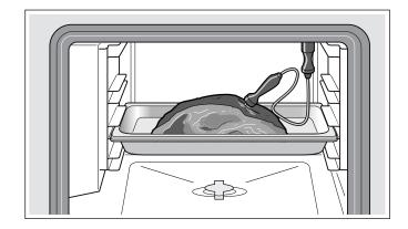
If there are several pieces of food, stick the core temperature probe into the middle of the thickest piece.
