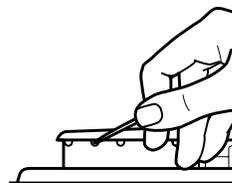
4. Replace the burner cap, making sure the alignment pins are properly aligned with the burner cap.
