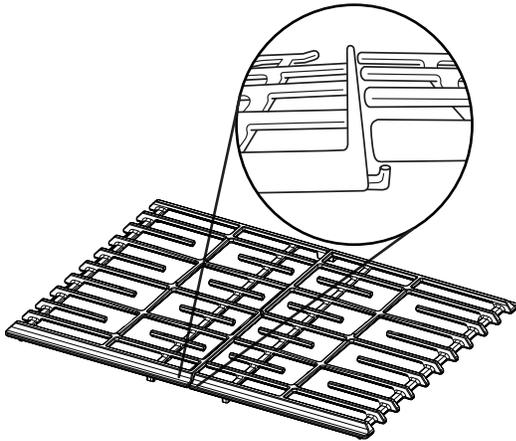
On some models, the two grates are identical and can be used on either the left or right side of the cooktop. Grates that are designed for use on only one side of the cooktop will have either "LEFT" or "RIGHT" embossed on the bottom side of the grate.
