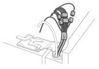
**4** Push the water supply tube into the hole on the top case and pull it through the backplate.
