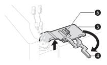
4 Lift the door from the middle hinge pin and remove the door.
