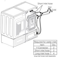
2. Front-loading washer and pedestal washer with Turbo Steam dryer
