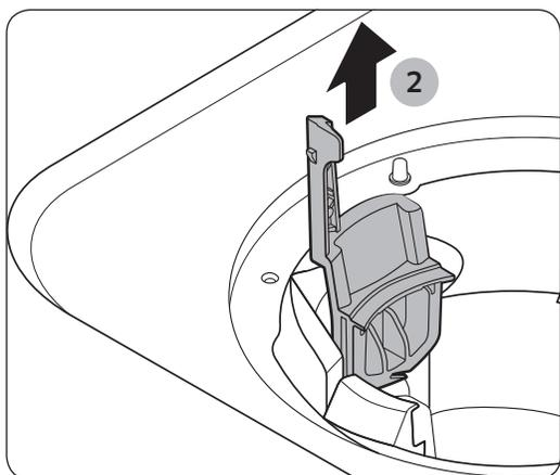
If the dishwasher fails to drain because the drain pump is clogged with foreign matter or there is an abnormal noise coming from the drain pump, you must unclog and clean the drain pump as instructed below.
