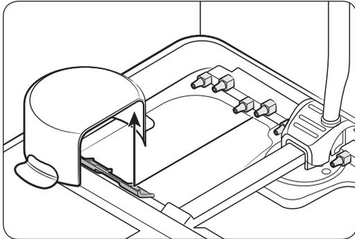
For more effective cleaning, load large items into the left side of the lower rack—the Zone Booster area. The Zone Booster function supplies more powerful water jets to the Zone Booster area. Make sure pot handles and other items do not interfere with the rotation of the nozzles and the water reflector.
