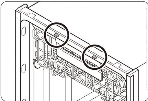
The Auto Release™ Dry function is designed to improve drying performance. It automatically opens the dishwasher's door 5 to 15 minutes before a cycle ends. You can use 2 methods to activate or deactivate this function.
