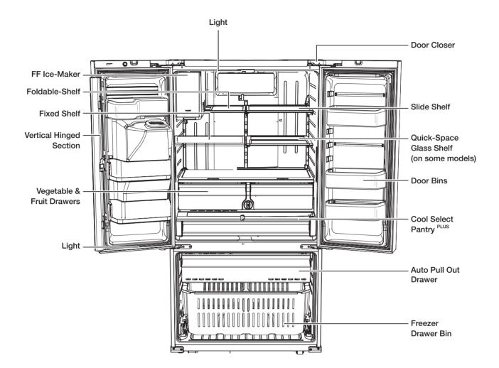
When closing the door, make sure the Vertical Hinged Section is in the correct position to avoid scratching the other door.
