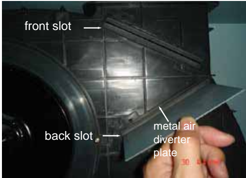
1. Remove air diverter plate slot covers. Remove metal air diverter plate from front slot and re-position to back slot. Re-install air diverter plate covers.
